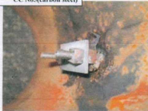
Fig.(4):Shows the installation of the Corrosion Coupon and Scale Coupon in Position No. 1(6 inch)
