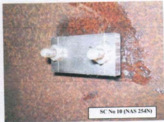
Fig.(9): Shows the installation of the Corrosion Coupon and Scale Coupon in Position No.6(10 inch)
